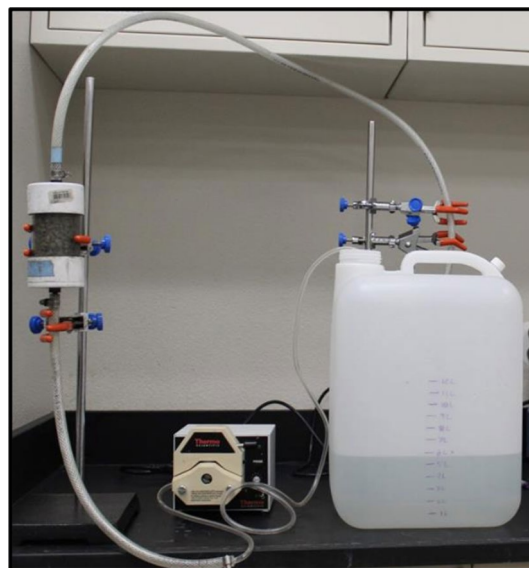
Fig. 5 Example of small-scale column experiment
