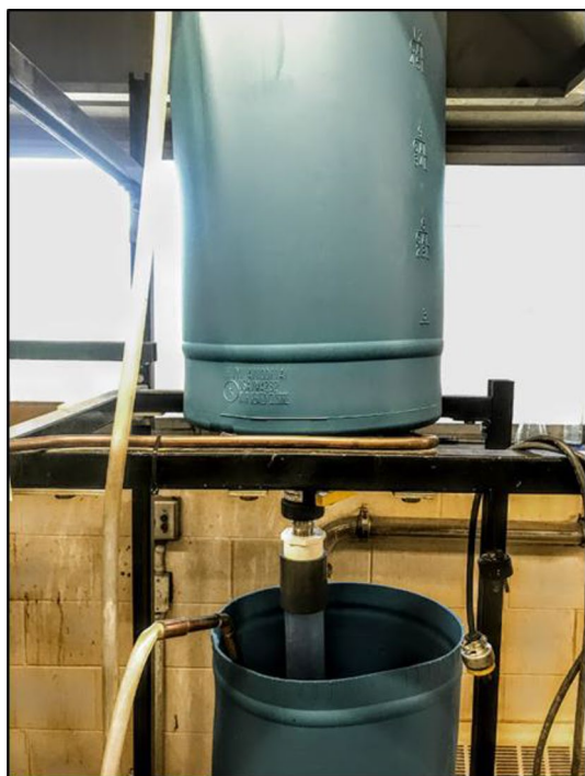
Fig. 4 Laboratory setup for permeability column experiments
