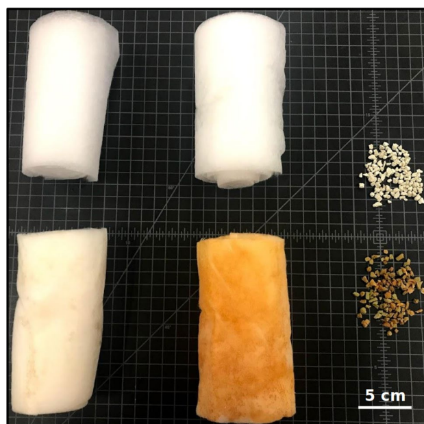
Fig. 9 Left to right: 12 g of Si, 12 g of Si+APTES, and 5.4 g of clinoptilolite before (top row) and after (bottom row) batch sorption experiments. Orange color is due to sorbed/precipitated iron (oxyhydr)oxides
