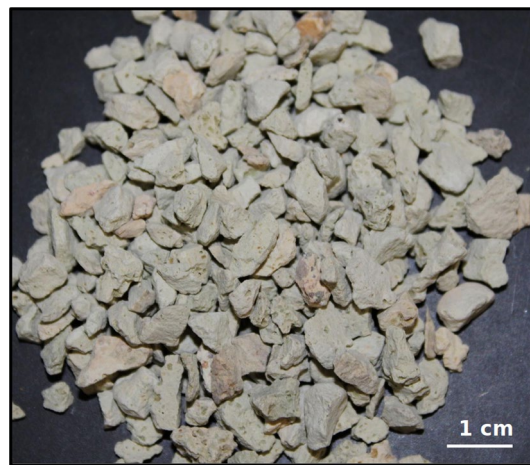
Fig. 3 Clinoptilolite grains, 2.4–4.8 mm diameter ( 4 \times 8 mesh)
